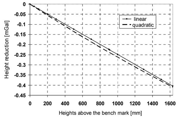
**Fig. 1.** Linear and quadratic functions of height reduction of gravity
