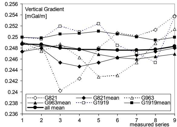
**Fig. 2** VG values by linear approximation from measurements at three different heights
