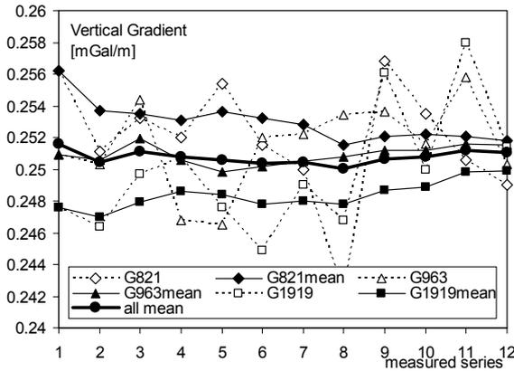
**Fig. 3** VG values and running mean height reductions referring to each gravimeter by linear approximation from measurements at four different heights
