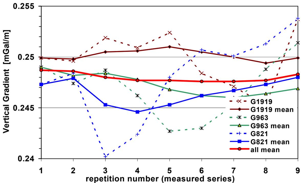
*Fig. 2. VG values by linear approximation from measurements at 3 different heights*
