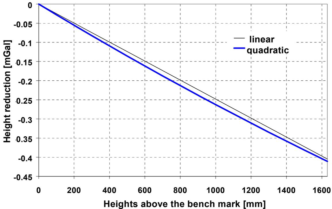
Fig. 1. Linear and quadratic function of height reduction of gravity
