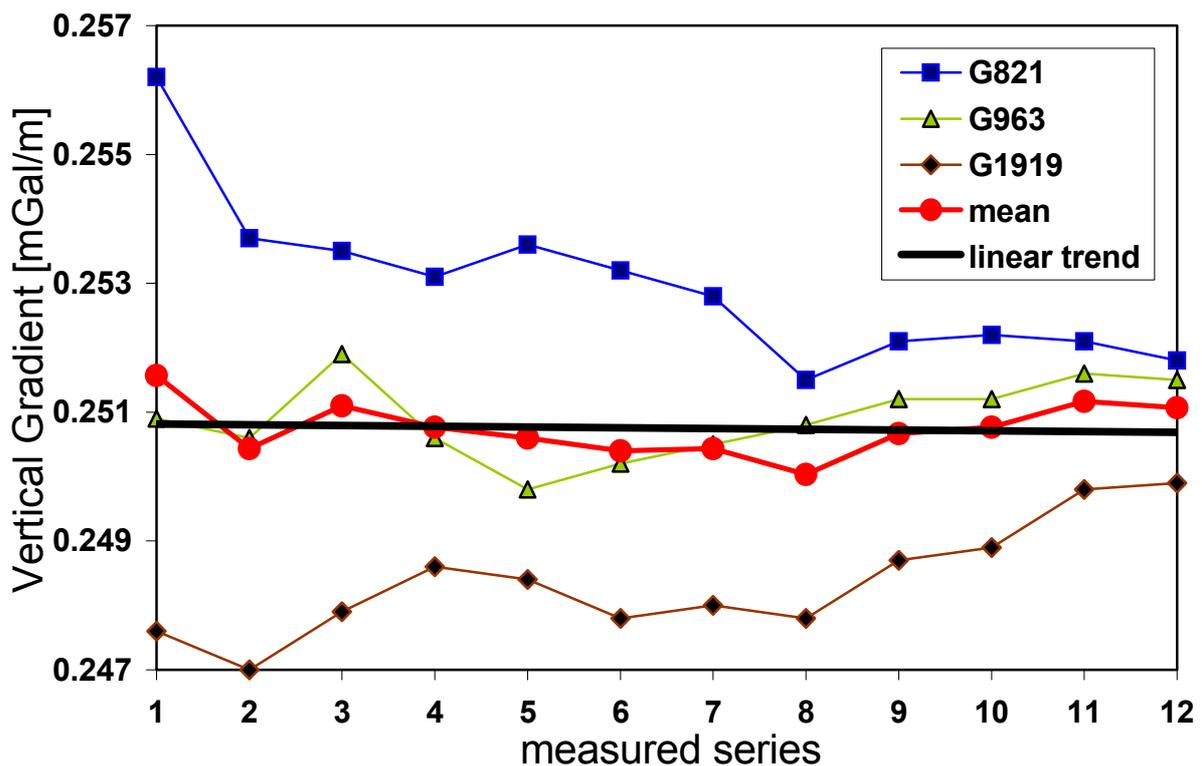
*Fig.4. Continuous mean values of VG referring to each gravimeters*
