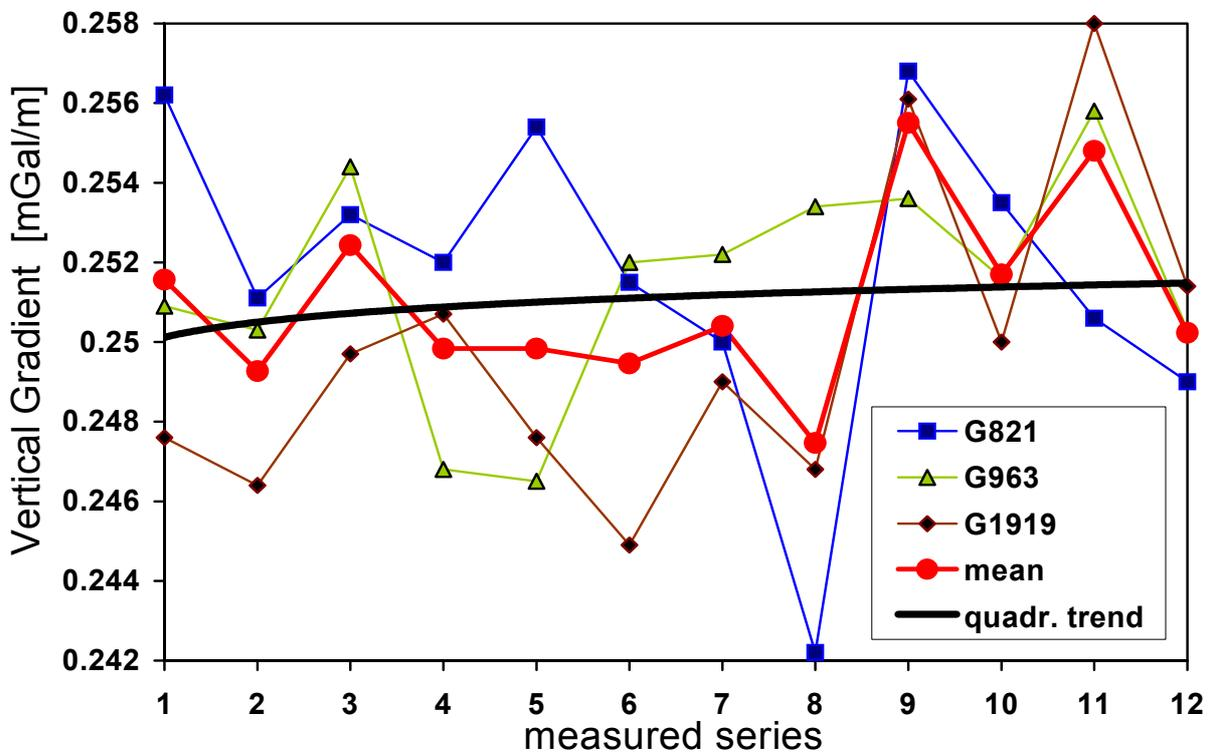
*Fig. 3. Values of VG by linear approximation from measurements at 4 different heights*
