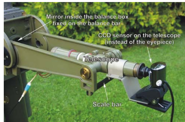
Fig. 3 CCD camera on the reading arm of the torsion balance
