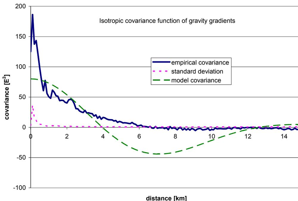
Fig. 2. Isotropic covariance function of gravity gradients
