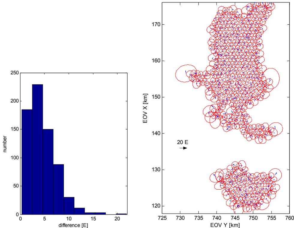
**Fig. 5.** On the left subfigure histogram of the deviations between measurements and predictions is shown (the mean deviation is 4.5 E). On the right subfigure one can find the vectors of prediction errors and three-sigma confidence ellipses for selected 700 torsion balance measurement sites.
