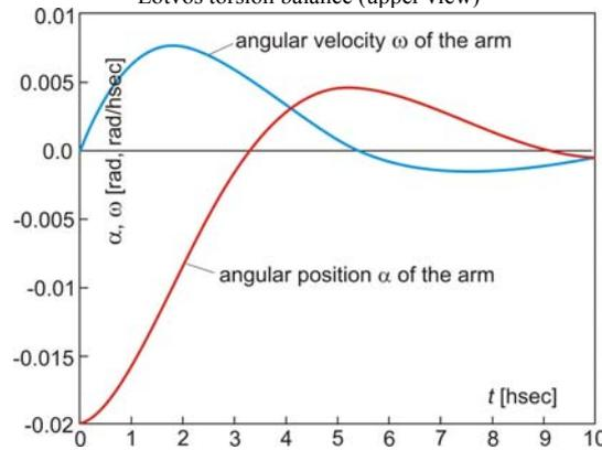
Fig. 8. Time-dependent angular position  $\alpha$  and angular velocity  $\omega$  of the torsion balance arm obtained by CFD modelling (time  $t$  is measured in hectoseconds, 1 hs = 100 s)
