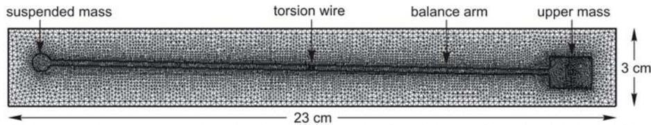
Fig. 7. Main geometrical parameters of the chamber and computational mesh for two-dimensional CFD modelling of the Eötvös torsion balance (upper view)
