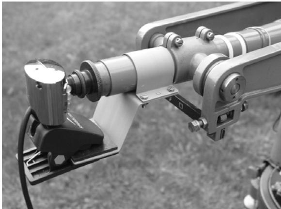
**Fig. 1.** Mounting of a CCD camera for automatized readout
