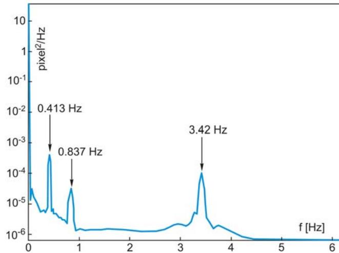
**Fig. 5.** PSD of time series captured by CCD sensor at 12.5 Hz sampling rate.
