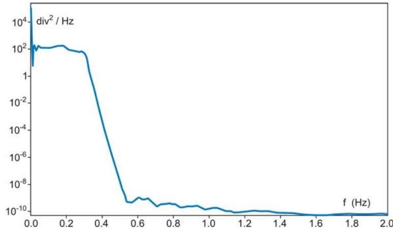
**Fig. 6.** PSD of time series of the balance marked as [] (square), captured in the first azimuth with 4 Hz sampling rate (div means scale division units)
