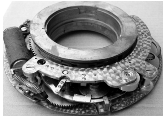
Fig. 3. The clockwork for turning the torsion balance
